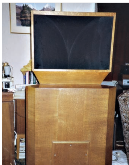
Fig. 1: A version of the Voigt HC Corner Horn which incorporated a bass chamber to give an extended low-frequency response. Reader Ken Whitfield from Wiltshire has two of these horns and they both require a really big room (see text).
