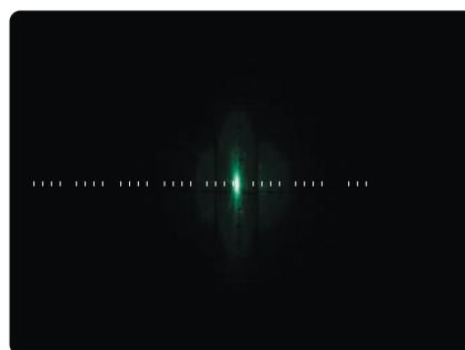
Fig. 2a: This example of astigmatism is caused by vertical elongation of the scanning spot, which is largely correctable by the front astig control. The spot is shown statically on the screen. As can be seen the vertical size is larger than the horizontal width. This state would indicate some form of astigmatism control is required (see text).
