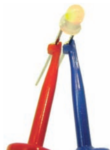
Fig. 4: The probes used on both units are of the wire-ended hook on type. (See text for comments).
