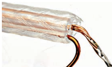
Photo 2: Close up view of the modified cable, showing the sensor wire inserted (solid copper wire shown curving into the air space).
