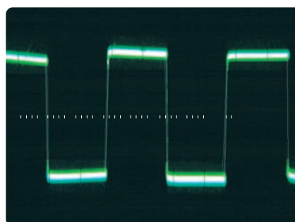
Fig. 2b: With the spot problems exhibited in Fig. 2a, the horizontal areas of signals become difficult to see in detail due to blurring. Note the effect shown on the tops and bottoms of the square wave shown here.
