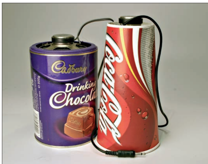
Fig. 1: Using a drinking chocolate or 'fizzy drinks' container to provide a resonant speaker cavity suitable for c.w. reception (see text).
