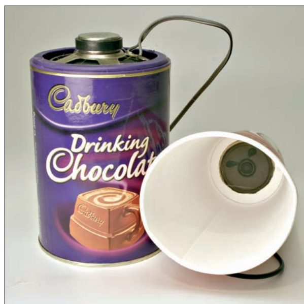
Fig. 2: Open ended and closed containers give different resonant frequencies. See text for more details.
